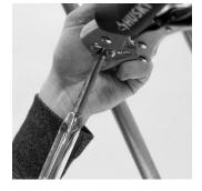
9. Using your T-bolt, add additional washers to reduce the clearance between the T-bolt and the bottom of the cup.
