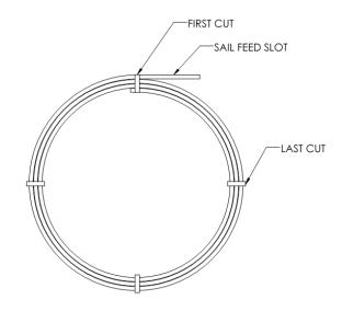
**UNCOILING THE LUFF EXTRUSION**
