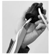
4. A) Using the de-cored (hollow) end of the halyard with the metal ferrule, pass the ferrule down through the slot at the top of the luff extrusion on the opposite end of the sail feed slot. Trimming the halyard to the correct length will happen once the entire furler is setup.
