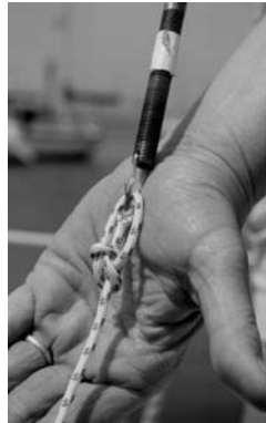
connecting swage stud to messenger line
