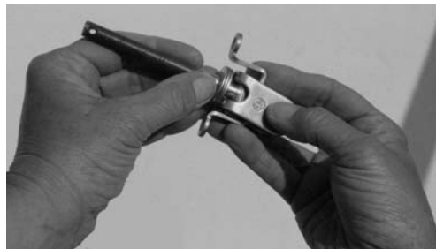
Adding washers to the T-bolt so the toggle will reach the chain plate hole
