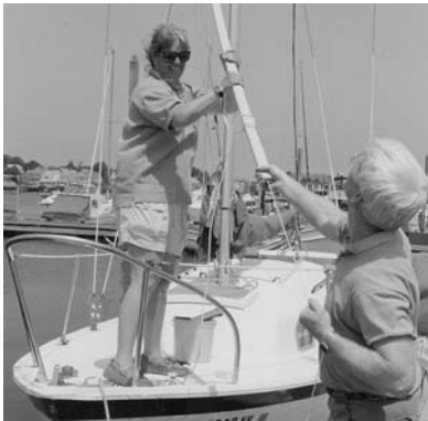
pushing extrusion up forestay
