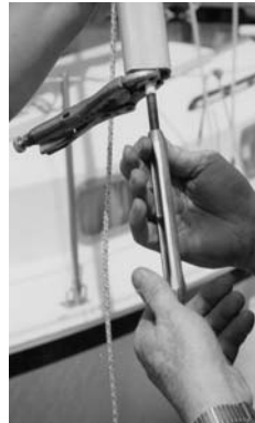
screwing turnbuckle on stud
