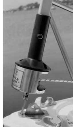
Furler w/ luff support pin installed
